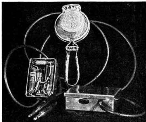
The interior of the single valve pre-amplifier can be seen on the left of the picture. The two-stage version is shown in its screening box to the right; the knob of the gain control protrudes through the slot in the side.
