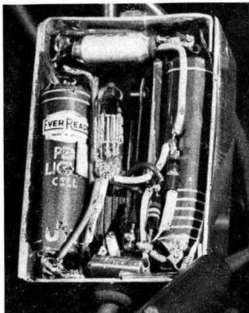
The interior of the single valve pre-amplifier showing the position of the major components.
